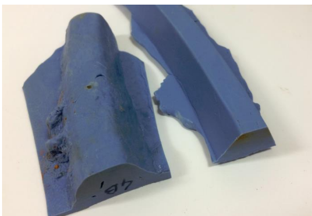
Fig. 29. Plasticine mould of the groove before repair (left) and after repair (right)
