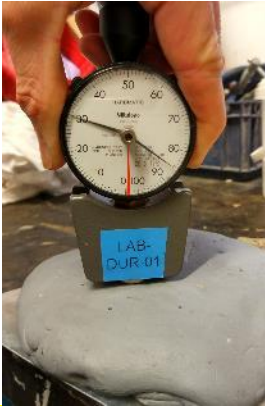
Fig. 13. Hardness measurement on F3XSS
