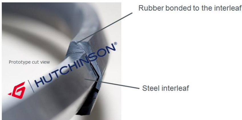
Fig. 8. Cut view of the hybrid gasket
