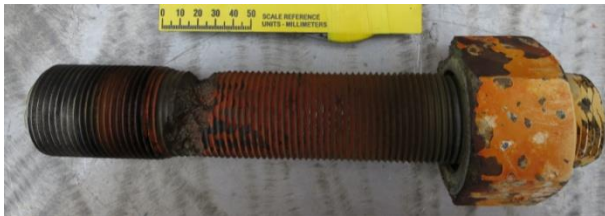
Fig. 22. Damage on a recovered stud (2inch diameter)
