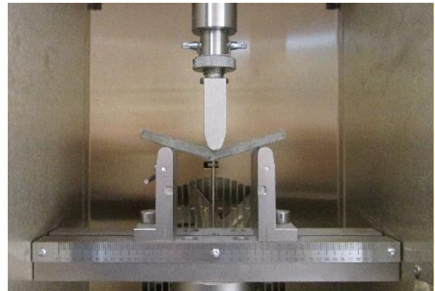
Fig. 16. Bending test ongoing
