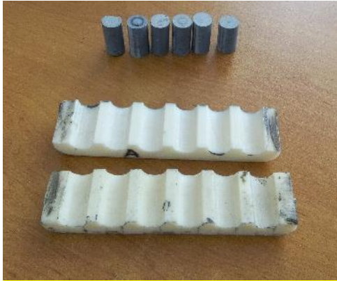
Fig. 18. Mould of the compression samples
